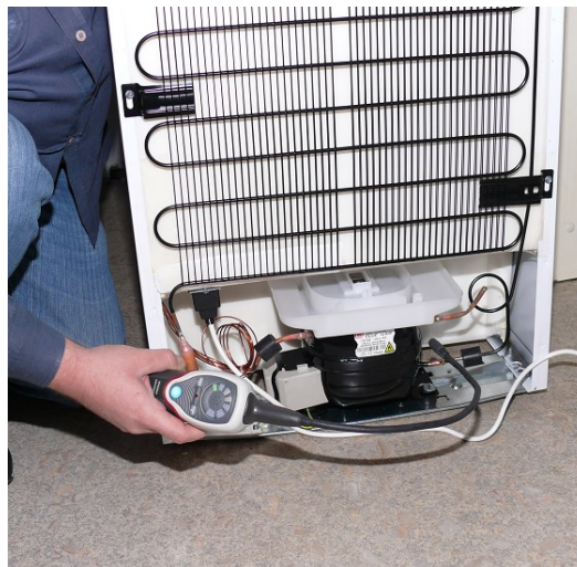
Figure FORStep1-3 Gas leak checks in a refrigerator
