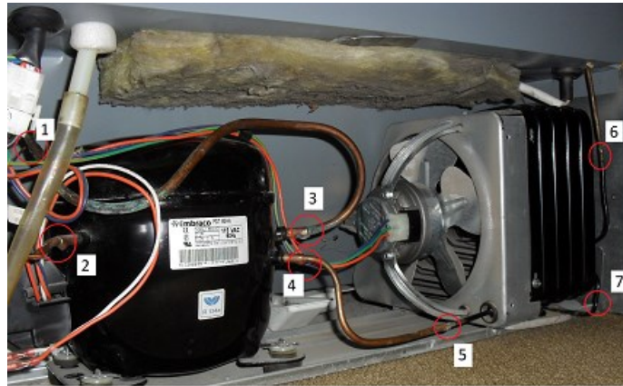
Figure FORStep1-2. Refrigerator system assembly. There are some connections between different parts of the system marked by numbers (1) – (7).
